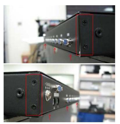
**Step 4:** Finally, please follow Step 3 to Step 1 to install back the rear kit, small cover & top cover to complete the procedure of replacement.
