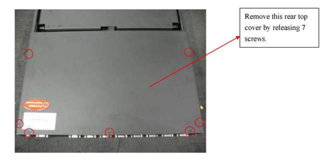
**Step 2:** Remove the small top cover behind the LCD panel.
